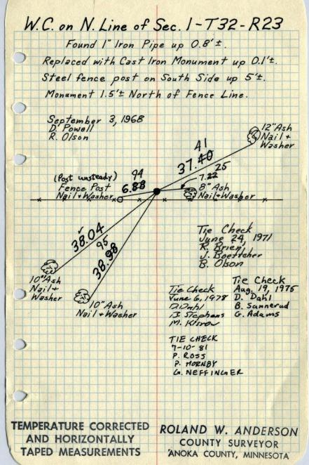
W.C. on N. Line of Sec. 1-T32-R23 Found I" Iron Pipe up . 0.8't. ). Replaced with C.I. Mon. up O.1't. Steel Fence Post on South Side up 5th Fence Pest 6.88 7.22 2 8" 10" Jsh 38.0 411 15/12
